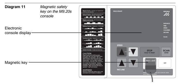
Before you can turn ON the treadmill, you must move the magnetic safety key to the ACTIVATE position on the electronic console. See Diagram 11. The treadmill's ON/OFF switch cannot be turned ON unless the safety key is in this position.
